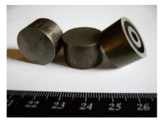
Figure 5. View of the experimental magnetic cores.
